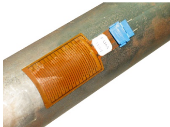
Picture: PowerAct vibration sensor and dampener; Source: http://ww1.prweb.com/prfiles/2008/08/12/416804/pa16nisopipe.jpg
